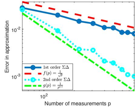
Fig. 1. Approximation error after using  $\Sigma\Delta$  quantization order 1 and 2 to quantize CS measurements of 4-sparse signals and reconstructing via the one-stage recovery method with 4-sparse signals. We also plot the graphs of  $f(p) = c_1 p^{-1/2}$  and  $g(p) = c_2 p^{-3/2}$  for comparison.
