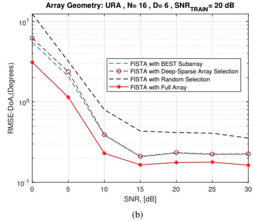
Fig. 1. Performance comparison of different antenna selection techniques with a URA geometry: (a) DOA estimation by applying MUSIC and (b) DOA estimation by applying FISTA; CNN-based antenna selection method gives 6 dB less error compared with random antenna selection. For a given antenna selection method, estimation accuracy of MUSIC is 5 dB better than that of FISTA.
