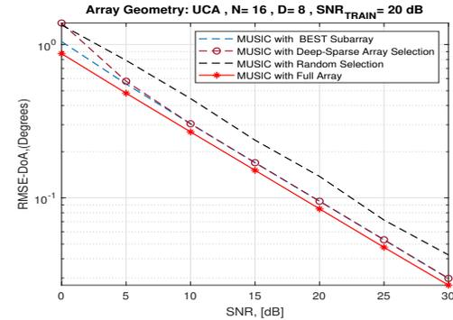
Fig. 2. Performance comparison of different antenna selection techniques with a UCA geometry with MUSIC technique based DOA estimation; CNN-based antenna selection method gives 6 dB less error compared with random antenna selection.
