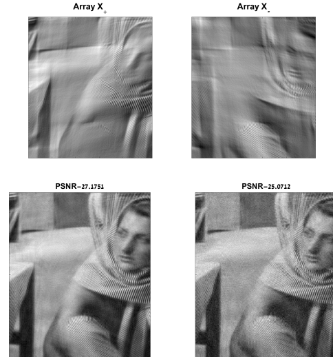
Fig. 6. Topt: Partially restored “Barbara” image by \mathbf{X}_+ (left) and \mathbf{X}_- (right). Bottom: Fragments of the image restored from directional (left) and TP (right) wavelet transforms
