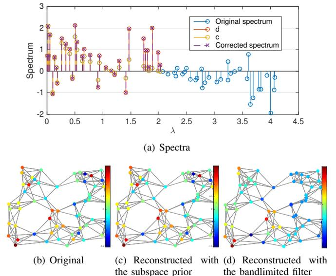
Fig. 3. Experimental results of signal recovery experiments. MSEs of signal recovery with the subspace prior and with the binary bandlimiting filters are  $3.20 \times 10^{-28}$  and  $2.04 \times 10^{-1}$ , respectively.
