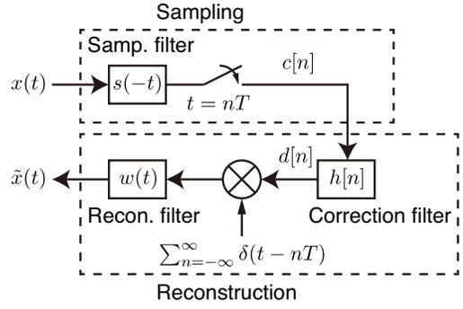
Fig. 1. Generalized sampling framework for SI spaces. The signals  $x(t)$  and  $\tilde{x}(t)$  are the original and reconstructed signals. The sequences  $c[n]$  and  $d[n]$  are the discrete-time samples and the corrected samples.
