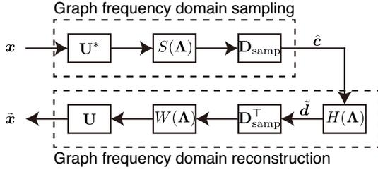
Fig. 2. Generalized sampling framework in the graph frequency domain.
